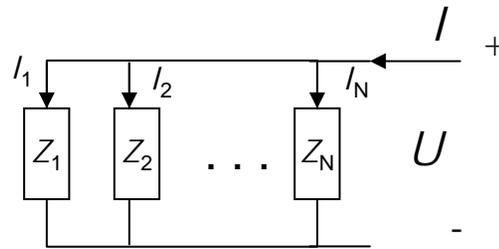
$$\left. \begin{aligned} I_1 &= UY_1 \\ U &= \frac{I}{Y_1 + Y_2 + \dots + Y_n} \end{aligned} \right\} I_1 = \frac{Y_1}{Y_1 + Y_2 + \dots + Y_n} I$$
