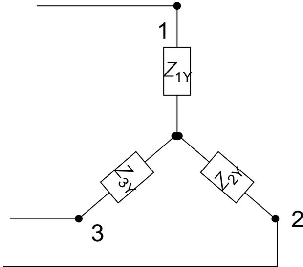
$$Z_{1Y} = \frac{Z_{2\Delta} Z_{3\Delta}}{Z_{1\Delta} + Z_{2\Delta} + Z_{3\Delta}} \quad Z_{2Y} = \frac{Z_{1\Delta} Z_{3\Delta}}{Z_{1\Delta} + Z_{2\Delta} + Z_{3\Delta}}$$
