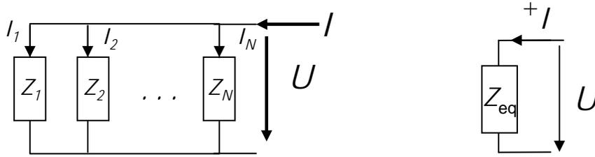
$$I = I_1 + I_2 + \dots + I_N = \left( \frac{1}{Z_1} + \frac{1}{Z_2} + \dots + \frac{1}{Z_n} \right) U = \left( \frac{1}{Z_{eq}} \right) U$$
