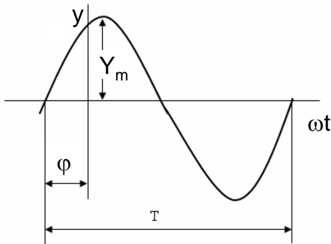
$$y(t) = \underbrace{\sqrt{2}Y}_{\text{amplitud}} \cos(\omega t + \underbrace{\varphi}_{\text{desfase respecto al origen}})$$
