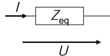
$$U = U_1 + U_2 + \dots + U_n = IZ_1 + IZ_2 + \dots + IZ_n = I(Z_1 + Z_2 + \dots + Z_n) = IZ_{eq}$$
