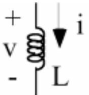
$$u(t) = L \frac{di(t)}{dt} \quad i = i(t_0) + \frac{1}{L} \int_{t_0}^t u(t) dt$$
