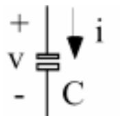
$$u(t) = u(t_0) + \frac{1}{C} \int_{t_0}^t i(t) dt \quad i(t) = C \frac{du(t)}{dt}$$
