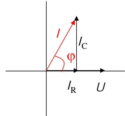
$$I_X = \frac{U}{jX} \begin{cases} \text{Bobina } I_X = \frac{U}{X_L} \angle -90^\circ \\ \text{Condensador } I_X = \frac{U}{X_C} \angle 90^\circ \end{cases}$$
